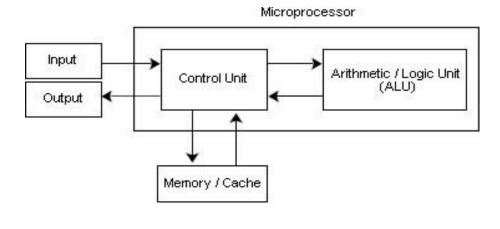
echnologies Parts of microprocessor
